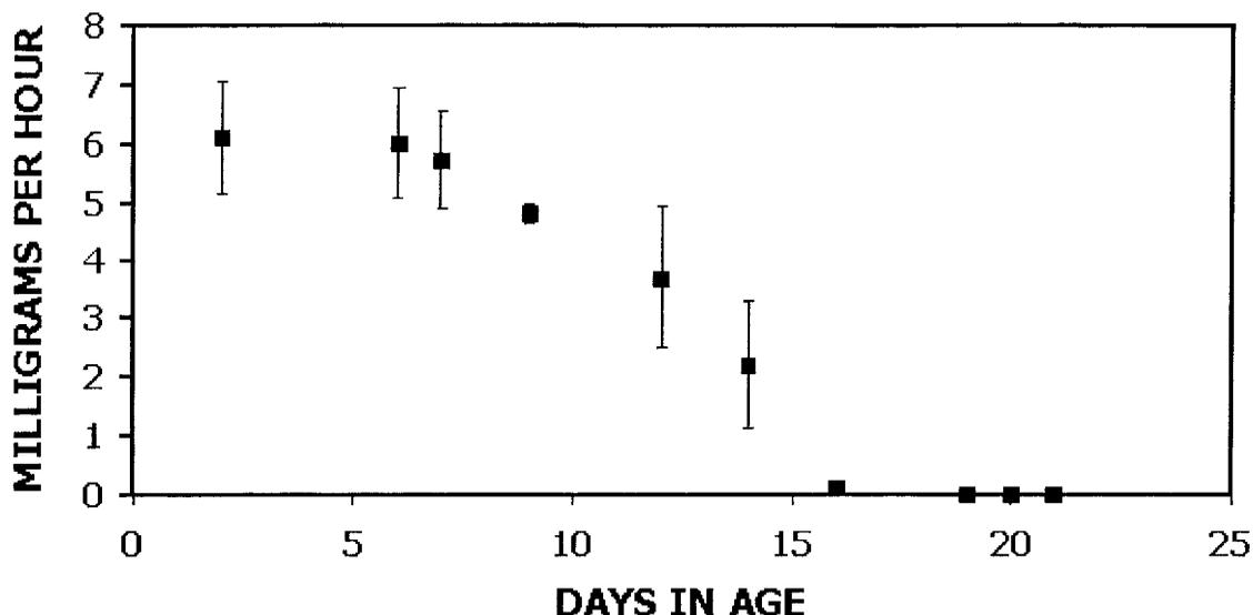
Fig. 2. Mean ( $\pm$ SE) milligrams of heptyl butyrate lost per hour from cotton balls in a laboratory fume hood. Cotton balls were soaked with 2 ml heptyl butyrate, and then were placed on aluminum foil weighing dishes.
