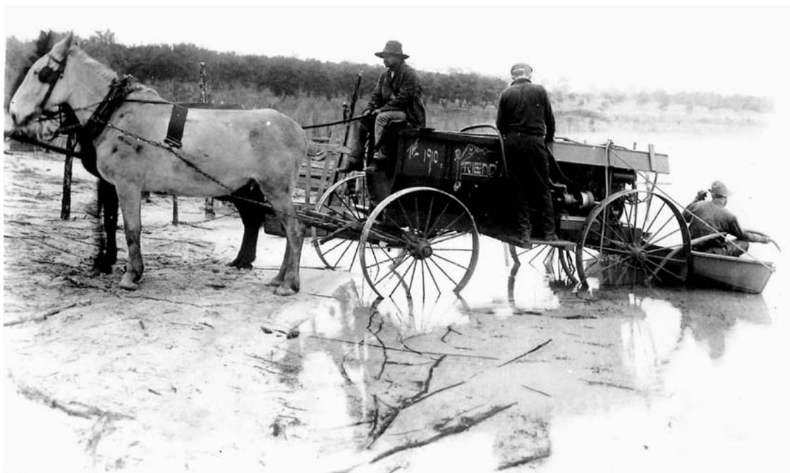
Fig. 7. Horse-drawn spray rig for spraying orange trees with experimental insecticides used by W. W. Yothers, about 1910. Yothers, in the boat at the right of the picture, is seen with a suction hose for obtaining water from the lake to fill the spray tank.
