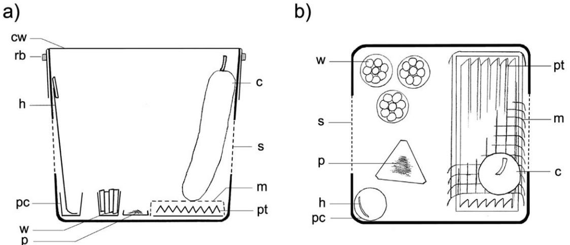
Fig. 1. Cross-section (a) and top view (b) of the prepared culture box. Legend: *c* = cucumber, *cw* = clingwrap, *h* = honey wick, *m* = metal mesh, *p* = pollen, *pc* = pill cup, *pt* = paper towel layers, *rb* = rubberband, *s* = silk windows, *w* = wet cotton rolls.
