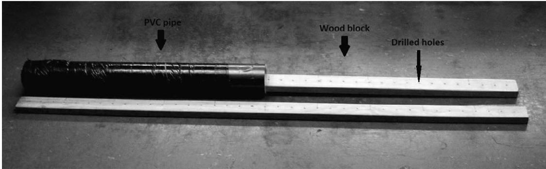
Fig. 2. Arena for negative phototaxis experiment. PVC pipe wrapped in black tape covered half of the wood block. Controls had no PVC pipe cover.
