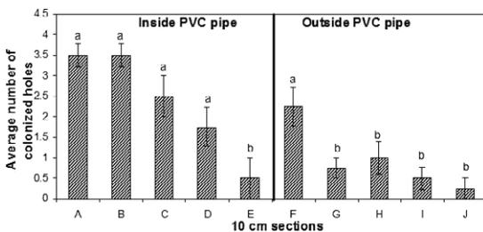
Fig. 4. Average number of *C. brevis* colonized holes per section ( $n = 175$ ). Sections A, B, C, D, and E were inside the PVC pipe and sections F, G, H, I, and J were outside the PVC pipe. Bars with the same letter were not significantly different at  $P < 0.05$ .
