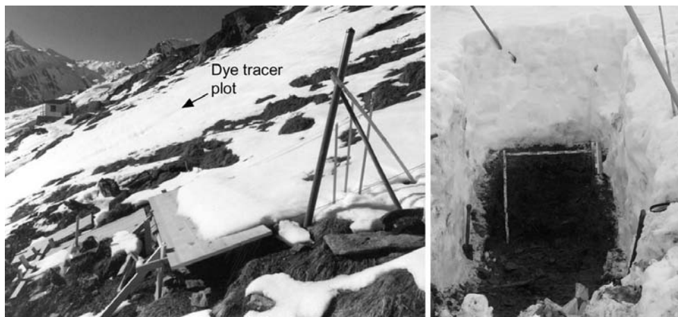
FIGURE 2. Left: View of the experimental site at Gd St Bernard, (2450 m a.s.l.) at the beginning of the winter. Runoff measurement installations in the front. Right: Example of an excavated profile on 14 May 2001 from which the flow pattern of the stained meltwater was analyzed.
