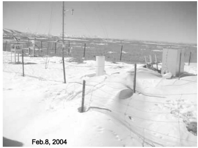
FIGURE 10. Snow cover trapped by the instruments and fence at the BJ site, in WSW direction.
