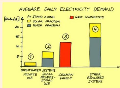
**FIGURE 6** Electricity demand drops when solar-electric stand-alone systems are used. An average private household consumes less than 3 kWh/d (1). Twice as much energy supplies 100 guests daily in a mountain lodge (2). The average German family supplied by the grid needs more than four times as much as a family using solar energy (3). Solar systems can also supply sufficient power for businesses or entire villages (4). (Graph by Fraunhofer ISE)
