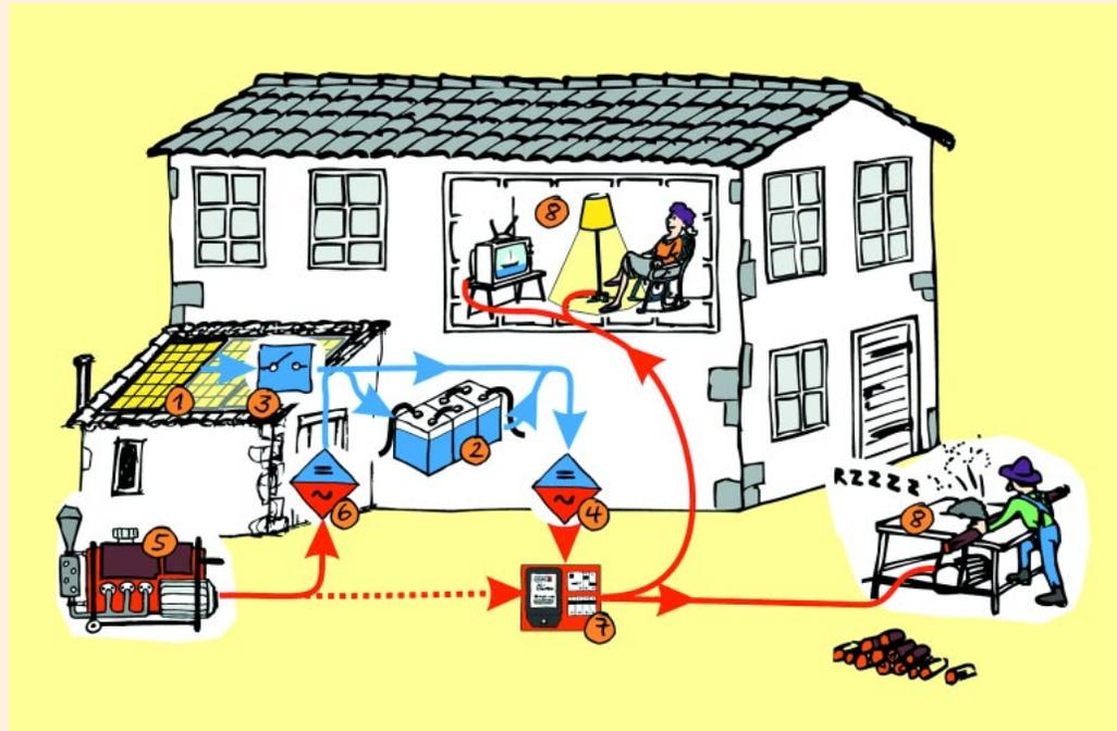
storage battery for use during times of less intense sunlight or at night. More advanced systems have a charge controller and/or an inverter that produces alternating current (AC) for electrical appliances designed to operate on this type of current. Larger systems, and those used in the Northern Hemisphere with lower seasonal insolation, often have an auxiliary energy provider such as a generator powered by a renewable source of energy (wind or water) or a diesel generator (Figure 2).
