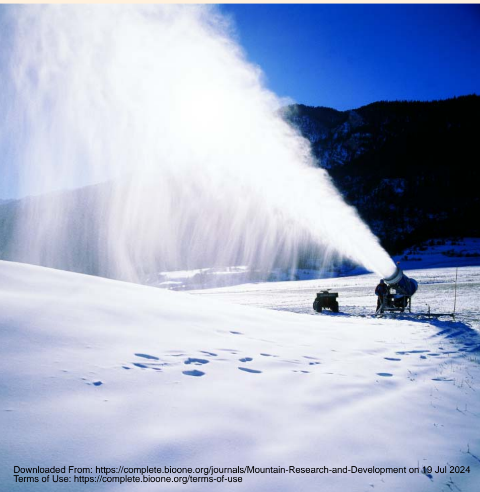
FIGURE 4 Snow cannon: such devices are expensive and can only be used under very specific climatic conditions. (Photo by Stefano Schröter, Keystone)
