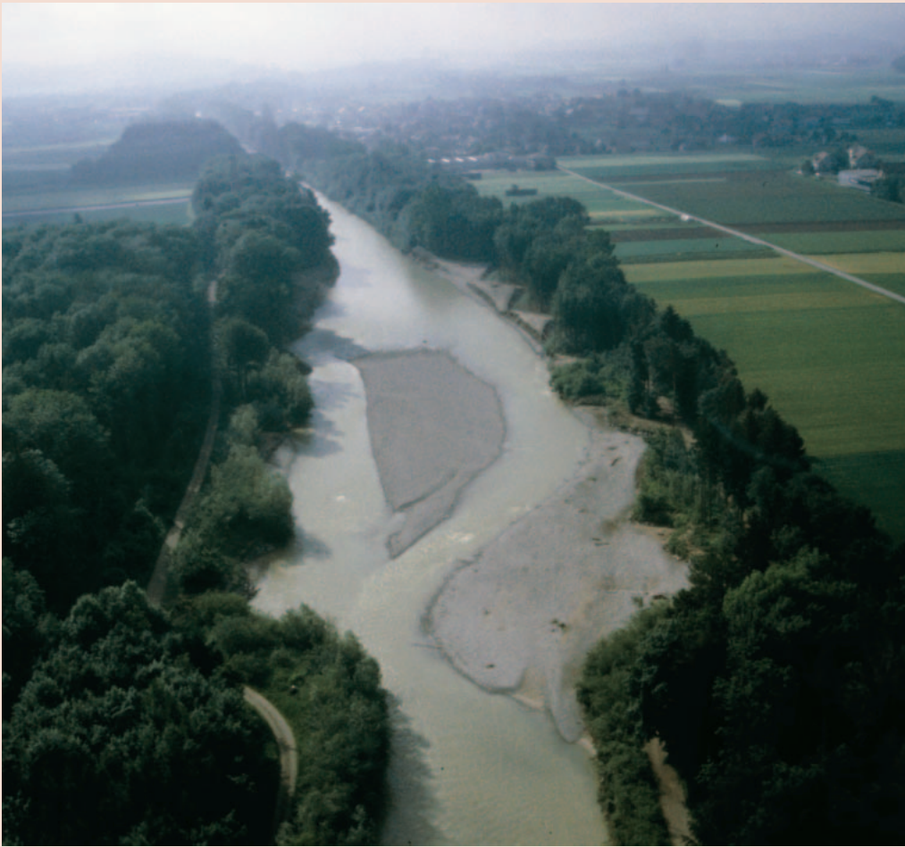
FIGURE 3 The result of a “Space for Rivers” initiative in Switzerland: the resilience of the Emme valley to flooding has been increased by allowing part of the Emme to return to its natural riverbed. This structural measure is cost-efficient, protects the river against undesired influx (thus improving water quality), helps conserve a natural ecosystem, and improves the quality of recreation areas. View of the Emme near Utzenstorf. (Photo courtesy of the Federal Office for Water and Geology, FOWG)
