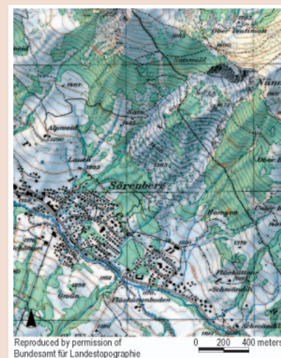
FIGURE 3 1993 topographic map, showing how the village has developed in the past 30 years in the area where debris flow formerly accumulated. (Map reproduced by permission of Bundesamt für Landestopographie, BA024084)
