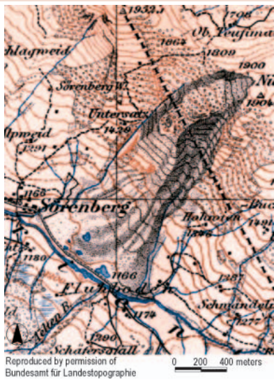
FIGURE 2 1918 topographic map, showing the open scars on either side of the mass and the typical accumulation features developed in 1910 and 1912. The few houses with the church (at the center of the village) are located in a safe place. (Map reproduced by permission of Bundesamt für Landestopographie, BA024084)
