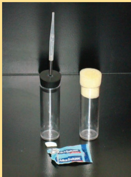
Figure 6. An alternative apparatus for initially anesthetizing Drosophila . Alka-Seltzer and 100 ml of water are added to culture tube on the left. The rubber stopper (with a hole into which a glass tube and pipet tip have been inserted) is placed over the culture tube. The CO 2 generated may be directed into a culture tube containing Drosophila .
