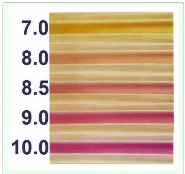
**Figure 1.** Photographs of low buffer salines containing 0.04 % m-cresol purple of indicated pH values perfused through PE10 tubing in the perfusion chamber used for the measurements with isolated and perfused anterior midguts of larval Aedes aegypti.
