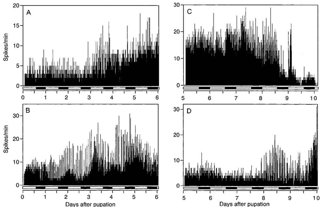
**Fig. 2.** Examples of long-term firing activities of labial cells in D-type males during the early (A and B) and late pupal periods (C and D). Photophase and scotophase are shown by white and black bars at the bottom, respectively.
