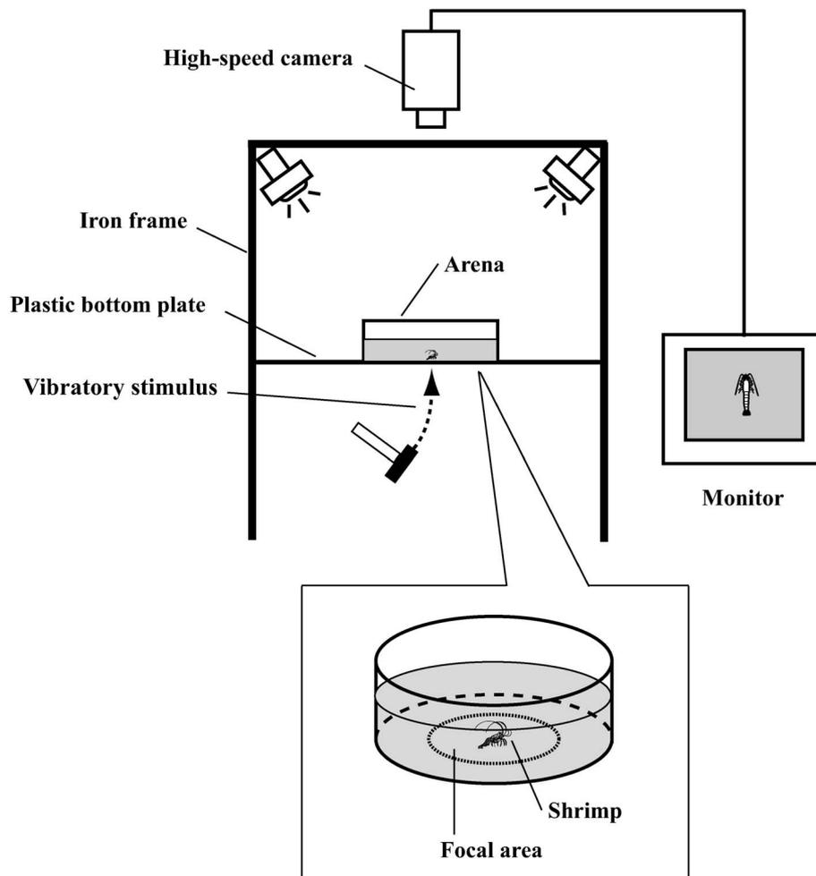
**Fig. 2.** Schematic diagram of the apparatus for observation of shrimp escape responses. Shrimp in the arena were stimulated with vibrations by striking the plastic bottom plate with a hammer from behind.
