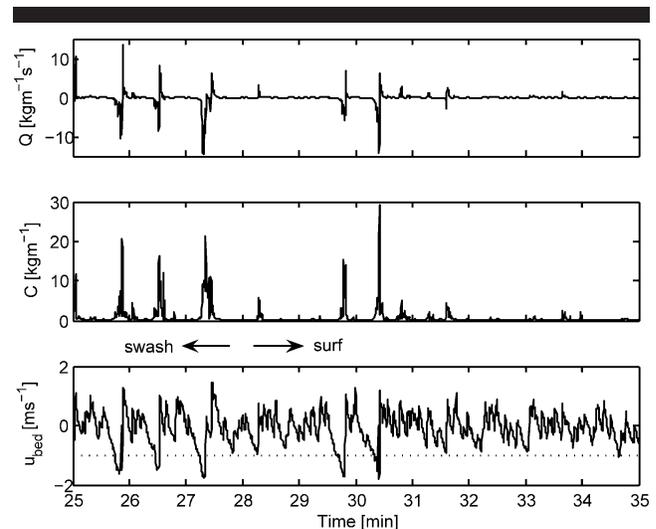
Figure 9. Swash/surf transition zone instantaneous time series. The dotted line in the lower panel represents an arbitrary velocity threshold, above which, large suspension events seem to occur.
