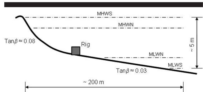
Figure 2. Beach profile showing rig position. MHWS = mean high-water springs; MHWN = mean high-water neaps; MLWN = mean low-water neaps; and MLWS = mean low-water springs.
