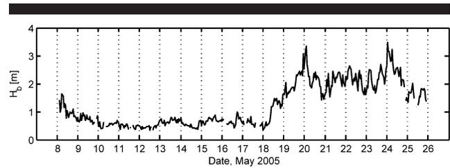
Figure 5. Time series of breaking wave height throughout the experiment. Dates on the x-axis correspond to 1200 on each particular day.
