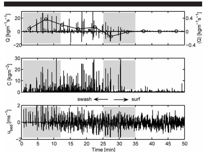
Figure 8. Time series showing where large sediment-suspension events start. The line with circles in the upper panel shows  $\langle Q \rangle$ . The grey areas correspond to the inner and outer expanded time series in Figures 9 and 10.
