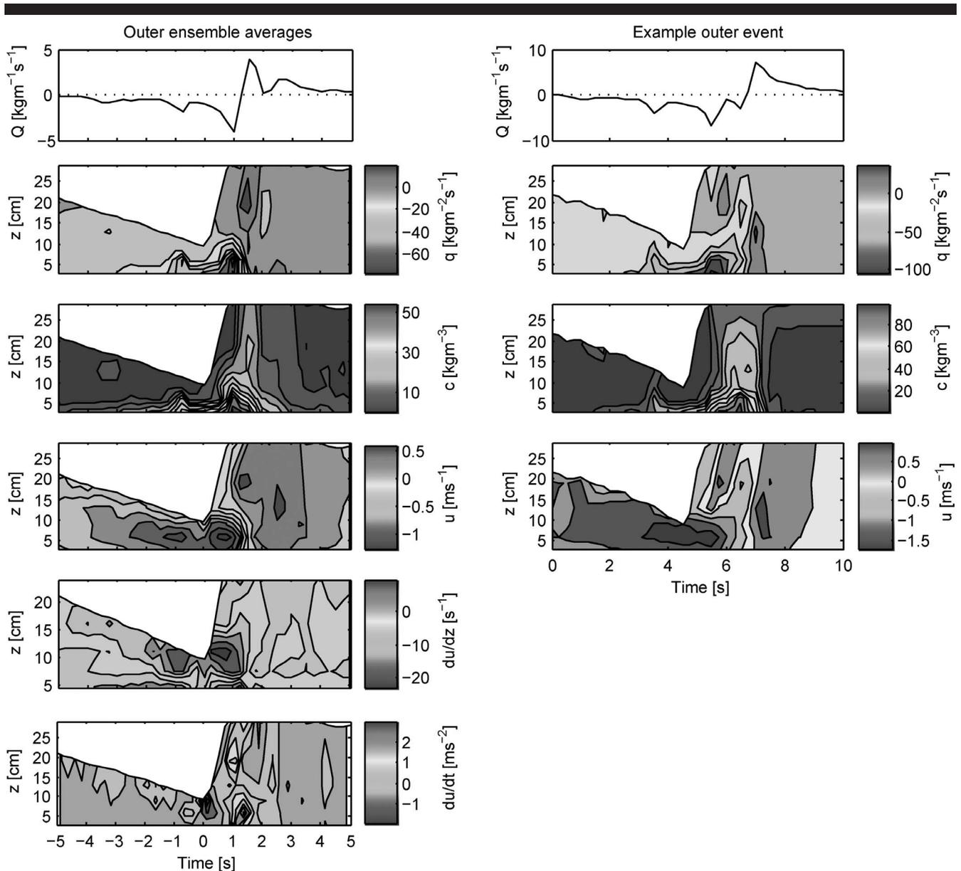
Figure 11. Ensemble-averaged (left panels) and example (right panels) events from outer-swash/inner-surf zone. On the ensemble average, time = 0 corresponds to the local minimum depth. **For a color version of this figure, see page 932.**
