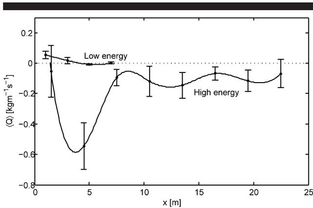
Figure 7. Sediment flux as a function of cross-shore distance, for low-energy and high-energy conditions. The original values of  $\langle Q \rangle$  have been removed for clarity. Each function extends from the shoreline to the approximate breakpoint.
