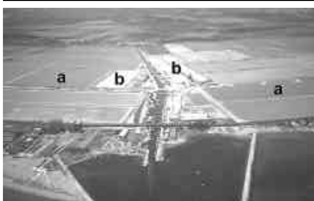
Figure 9. Aerial view of the Margherita di Savoia saltworks; in the foreground the evaporation ponds (greyish surfaces) and the big salt piles (white surfaces) can be observed. The harbour extension works modified the longshore sediment drift.
