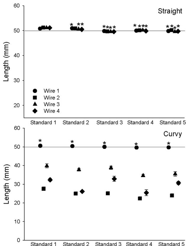
**Fig. 4.** Mean length (mm) for Layout A (straight) and Layout B (curvy) wires using Method 2. Standards 1-5 represent wire thickness from 0.65 to 0.15 mm. Specific wire orientation can be referenced in Figs. 1 and 2. Wires with asterisks were not significantly different than the expected length of 50 mm, indicated by the line.
