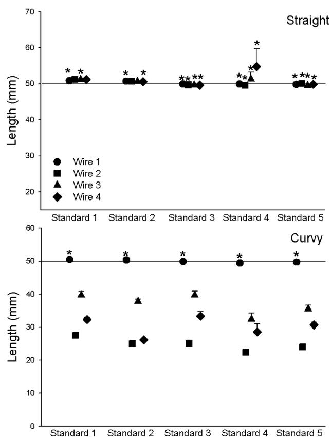
**Fig. 5.** Mean length (mm) for Layout A (straight) and Layout B (curvy) wires using Method 3. Standards 1-5 represent wire thickness from 0.65 to 0.15 mm. Specific wire orientation can be referenced in Figs. 1 and 2. Wires with asterisks were not significantly different than the expected length of 50 mm, indicated by the line.
