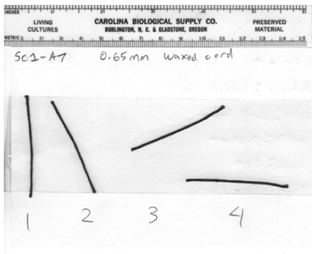
**Fig. 1.** Sample scan of a straight wire card (Layout A). This card has wire samples from Standard 1 (0.65 mm). Wire orientations moving across the card from left to right were: Wire 1 (Vertical), Wire 2 (~ 65 degrees), Wire 3 (~ 35 degrees), and Wire 4 (Horizontal).
