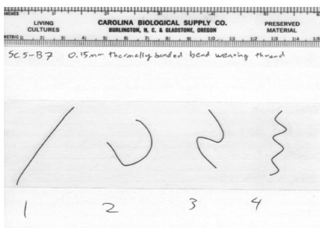
**Fig. 2.** Sample of a curly wire card (Layout B). This card has wires from Standard 5 (0.15 mm). Within Layout B the first wire is straight, but the remaining wires exhibit varying degrees of curvature, the second wire is "U-shaped", the third wire is "S-shaped", and the fourth wire is "curly".
