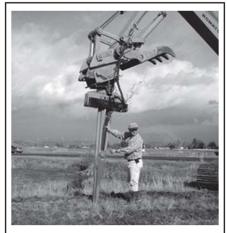
Figure 9. Long tube stock can be planted using an expandable stinger attachment for an excavator.
