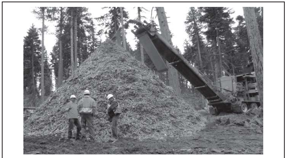
Figure 3. Grinding woody debris from slash piles to be used as mulch.
