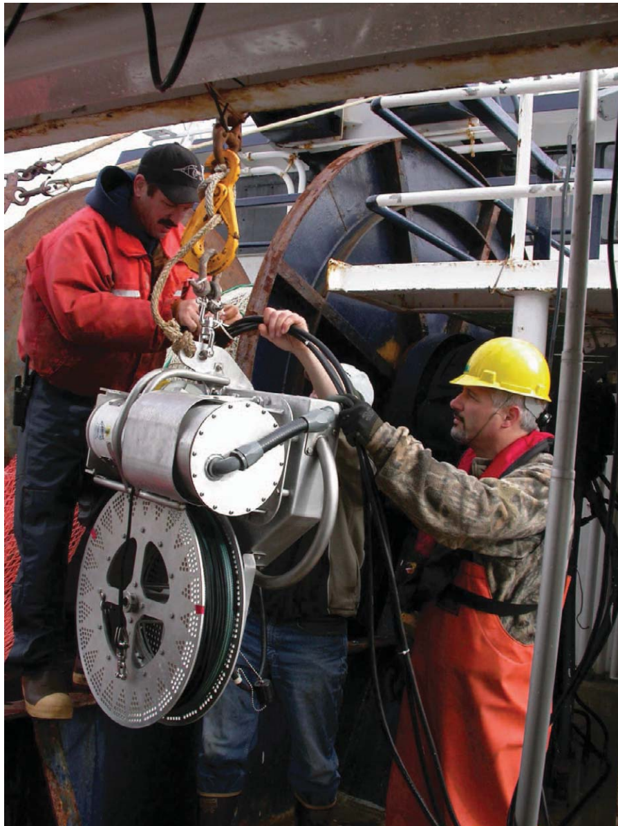
FIGURE 2. Photograph of the Sidewinder block winch showing the aluminum housing of the drum below the (left to right) planetary reducer, brake, line guide, and motor and the lifting handles above.
