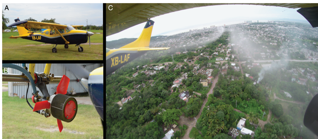
Fig. 2. (A) Aircraft employed in the trials with (B) the rotary atomizer mounted under wing and (C) aerial view during the application.
