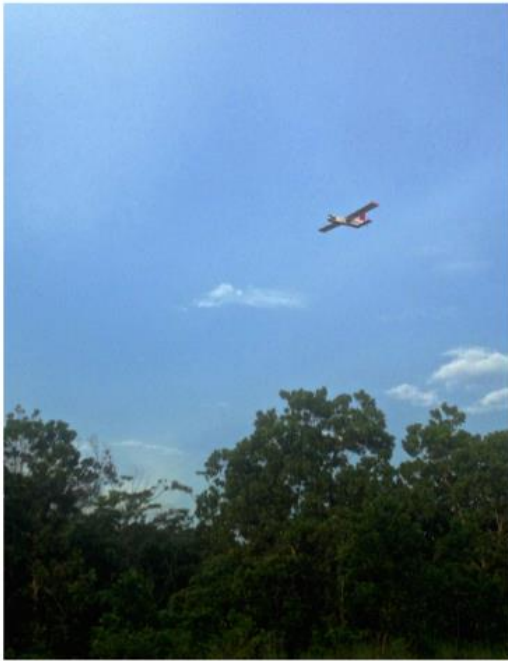
Fig. 3. The Unmanned Aerial Vehicle (aka “drone”) in action. These remote control planes have a flight range of about 40 km and are armed with a 12 megapixel digital camera. Through an auto-pilot they can be programmed to systematically survey an area of canopy. Photos can be stitched and analysed to produce a map of forest conditions.
