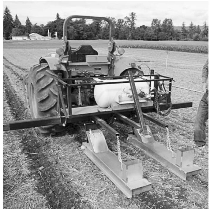
Figure 5. Two-row flame weeder designed by C. Merfield. Flame is confined to the crop row with row covers, and micro jets deliver water/organic herbicide in a curtain in front of the flamer to minimize the potential of the residue to ignite.
