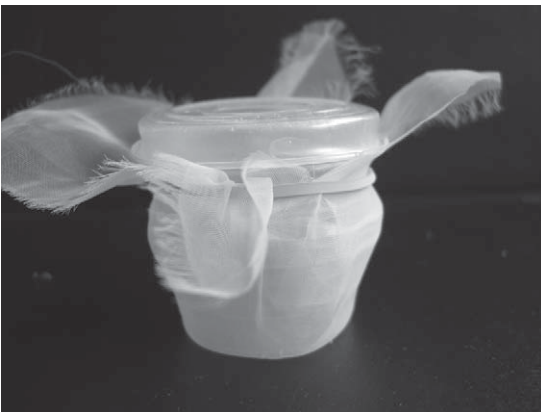
Fig. 2. Assembled Myzus persicae feeding chamber.
