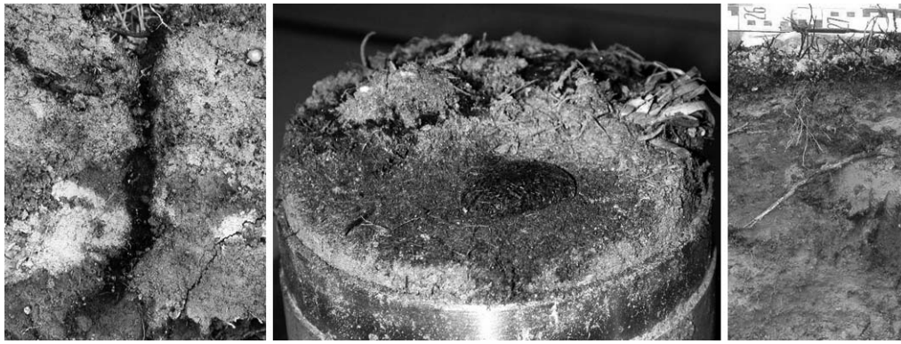
FIGURE 6. Triggers for preferential water infiltration observed at Hannigalp. Left: An ant channel with an extraordinary dye tracer concentration. Center: High water repellence of the soil surface, determined with the water-drop penetration method. Right: Roots of an Ericaceae shrub acting as a dominant water flow path from which the stained water spreads out to the adjacent pores.
