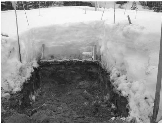
FIGURE 1. Top: View of the experimental site at Hannigalp (Grächen, 2100 m a.s.l.) shortly after the end of the snowmelt. Bottom: Example of an excavated profile on 30 April 2001 from which the flow pattern of the stained meltwater was analyzed.
