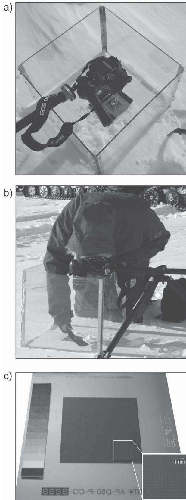
FIGURE 3. Field implementation of the instrumentation for using the DSPP method. (a) The fixed camera and the sample glass underlain by a dark reference plate to improve contrast; (b) example of surface snow sampling for photography; and (c) the micrometer accurate dot grid used. It is here equipped with a gray scale for light condition comparison.
