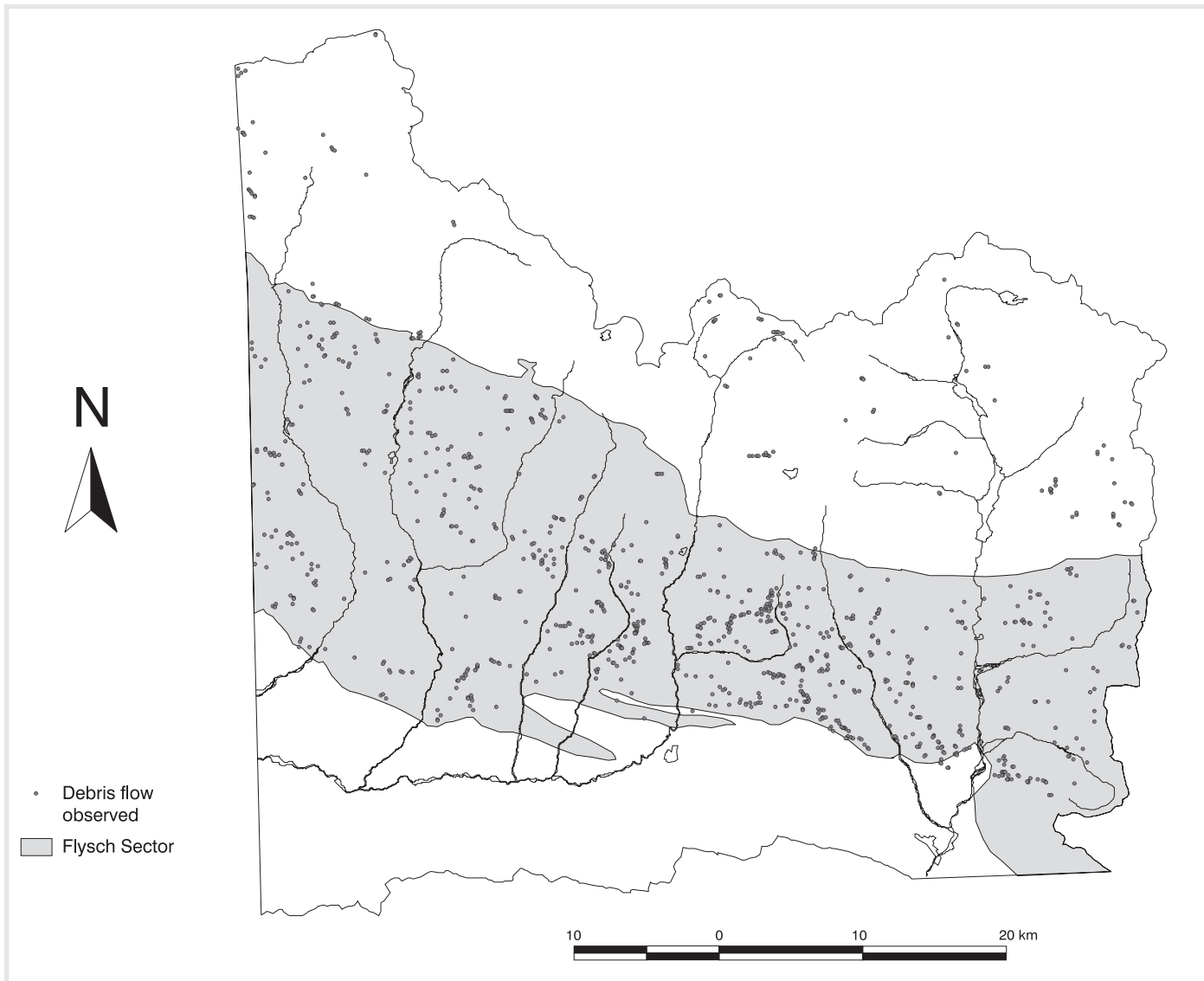
FIGURE 4 Location of hillslope debris flows in the Upper Aragón and Gállego valleys, with special reference to the Flysch Sector. Each dot represents the location of a debris flow scar. (Map by authors)
