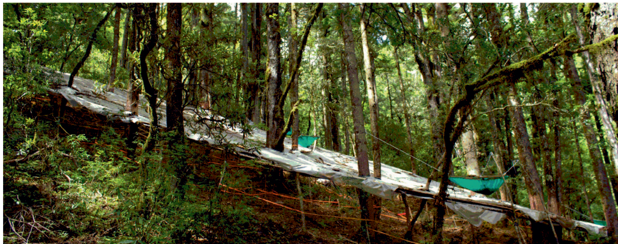
FIGURE 5 Experimental manipulation of precipitation using temporary plastic roofs (top) resting on 1–1.5 m bamboo poles (middle). Upslope of the roofed plot, a trench (bottom) was dug to prevent interflow of water.
