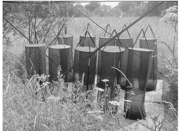
Fig. 2. The experimental layout showing the 10 insect cages; 1 microsward was placed on the ground in each cage.
