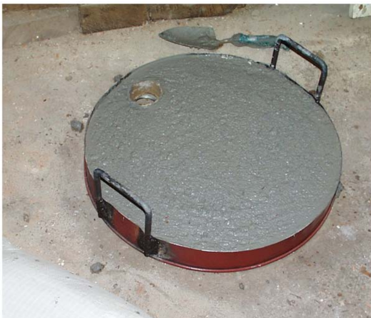
Figure 2. The kiln lid filled with sand/fireclay mixture, before drying and firing.
