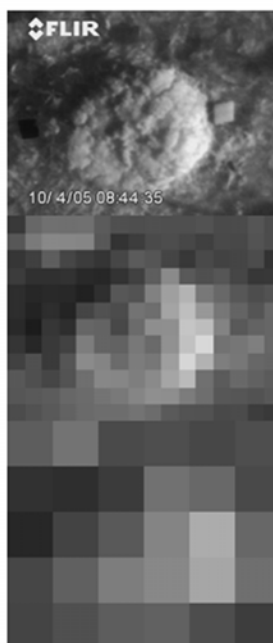
Figure 6. Thermal infrared image of a fire ant mound. Original image at 0.5 cm resolution (top); resampled image at 0.1 m resolution (center), and resampled image at 0.25 m resolution (bottom).
