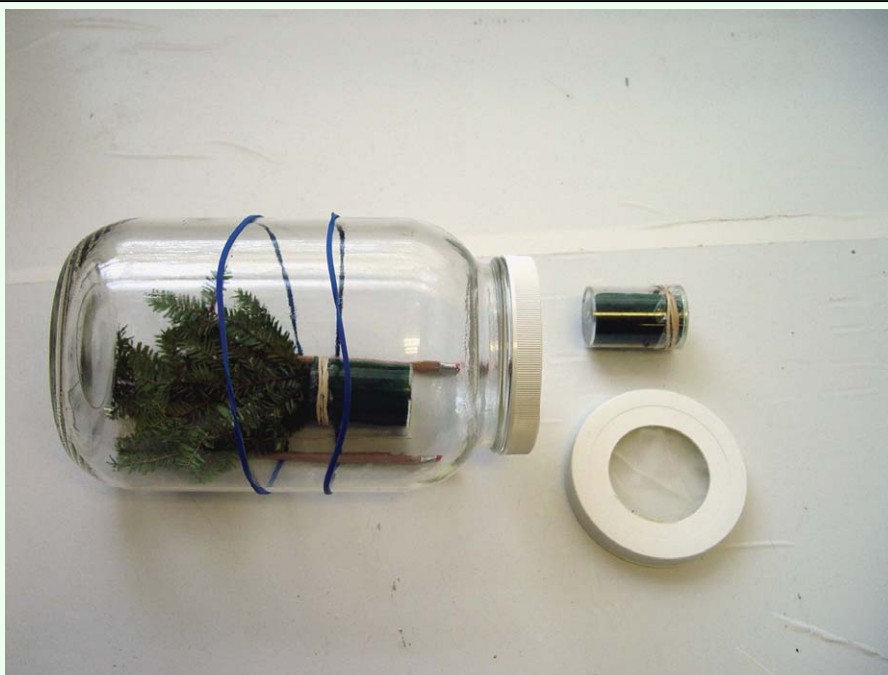
Figure 1. Glass (3.8 L) oviposition jar used in mass rearing Sasajiscymnus tsugae at Clemson University's insectary (Clemson, SC). Assembled jar shown at left, with hemlock bouquet inside, rubber bands holding two pencils underneath to prevent rolling, and lid in place. Plastic vial (6 cm tall x 4 cm diam) to hold the bouquet is shown at upper right, ventilation detail in lid shown at lower right. High quality figures are available online.
