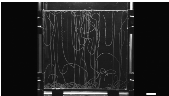
Fig. 3. Trajectories of planulae swimming in a narrow upright chamber (200 mm wide \times 3 mm deep \times 200 mm high) for 10 minutes. Scale bar, 20 mm.
