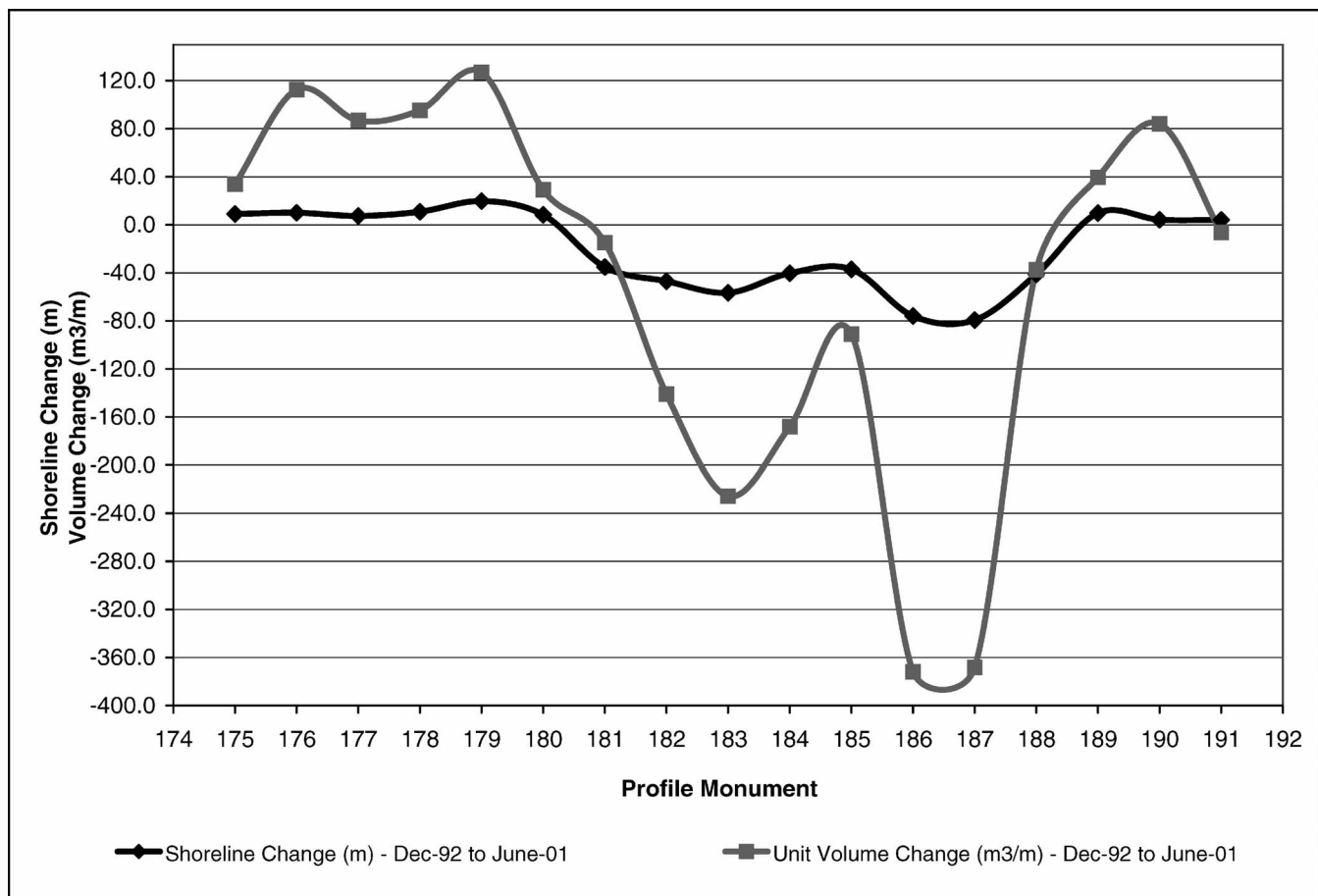
Figure 3. Shoreline changes (m) and volume changes ( \text{m}^3 \text{m}^{-1} ) from the postconstruction survey (December 1992) to the last survey of the entire study area (June 2001).
