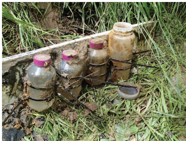
Figure 2. Photograph of peeper assembly.
