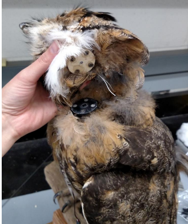
Supplemental Figure 1. Photograph demonstrating the two connector plates containing magnets for attachment of the mechanical lure owl head. The magnets allow for the head to fall off easily if struck by an attacking raptor during trapping efforts.
